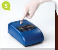
Blank measurement max. 20 seconds. Add the FOBreagent by pressing down the inner part of the cap.
