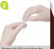
Remove the foil cover from the cuvette. The liquid surface should lie between the two lines marked on the cuvette. Do not touch the clear flat surfaces in the lower part of the cuvette.
