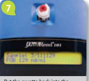
Put the cuvette back into the measurement well. The FOB result is displayed within 1 minute.
