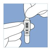
Remove the foil cover from the cuvette.
