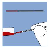
Pill the blue striped capillary with the sample (20 μL) up to the white stopper. Ensure that there are no air bubbles in the capillary. Wipe away any residual sample from the outside of the capillary.
