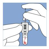
Place the sample  $(20~\mu L)$  into the buffer solution in the cuvette and dispense by pressing down the plunger. Make sure that the capillary is completely empty.
