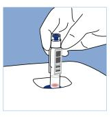
Insert the cuvette in to the measurement well of the instrument. The barcode should be facing you.
