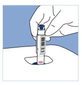
6 Insert the cuvette in to the measurement well of the instrument. The barcode should be facing you.
