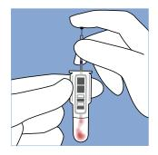
Place the sample (20 µl) into the buffer solution in the cuvette and dispense by pressing down the plunger. Make sure that the capillary is completely empty.
