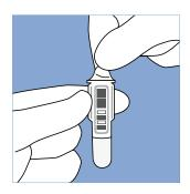
Remove the foil cover from the cuvette.
